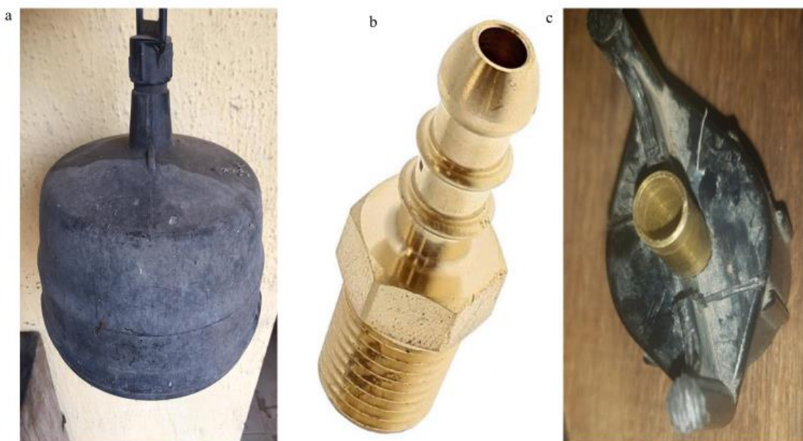
Figure 1. Images of a) digester vessel, b) gas pipe connector, and c) removable manhole cover.
